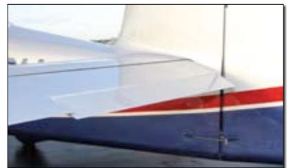
Electric pitch trim comes via a simple flap on the left elevator.
