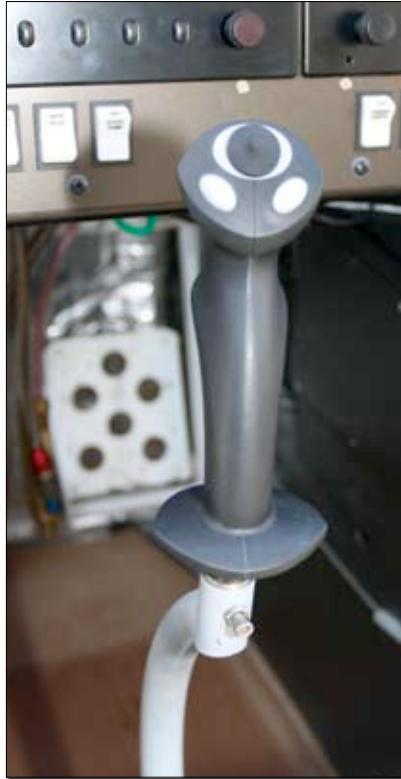
A Tosten stick grip includes trim, plus buttons for the flap motor, the coffee machine, ejector seats and push-to-talk.
