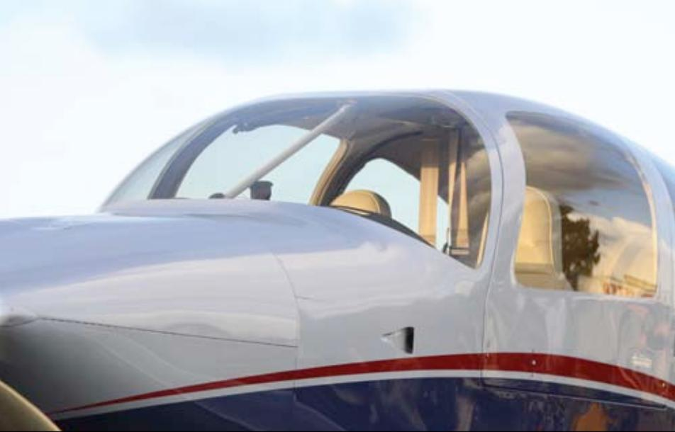
A sloped cowl and high upper corners of the windshield help create excellent visibility for the pilot. Note the steel-tube cabin reinforcement; the RV-10 was tested to stringent rollover standards.
