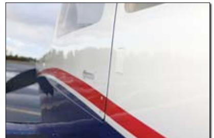
The overhead doors have not been trouble free. A recent factory service bulletin instructs owners to install a supplementary latch to keep the doors from leaving the airplane in the event that they come unlatched during flight.
