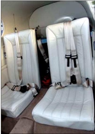
Split back seats can be removed to increase cargo capacity.
