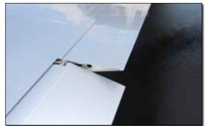
Tight-fitting control surfaces help aerodynamic efficiency. Great care in surface size, hinge placement and control geometry guarantee excellent handling qualities.
